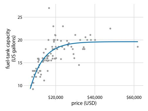
Fuel-tank data represented with an explicit analytical model. The solid line corresponds to a least-squares fit of the formula y=A–B exp(–mx) to the data. Fitted parameters are A=19.6, B=29.2, m=0.00015.
