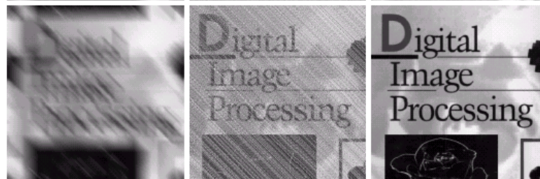
FIGURE 5.29 (a) Image corrupted by motion blur and additive noise. (b) Result of inverse filtering. (c) Result of Wiener filtering. (d)–(f) Same sequence, but with noise variance one order of magnitude less (g)–(i) Same sequence, but noise variance reduced by five orders of magnitude from (a). Note in (h) how the deblurred image is quite visible through a “curtain” of noise.
