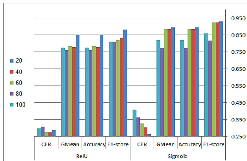
Figure 3. Sensitivity results over the ReLU and sigmoid activation functions using different numbers of hidden neurons.
